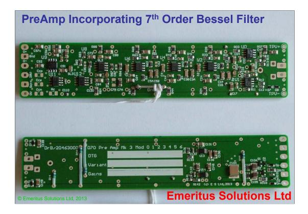
The PEC is the 54 dB Bessel filter fitted pre amplifier described in this presentation. The PEC only requires cable termination and potting to prepare it for use underwater. The surface mounted MLCC capacitors are of course an important enabling technology. The use of PU encapsulation requires all components to be suitable for use at ambient pressure.
